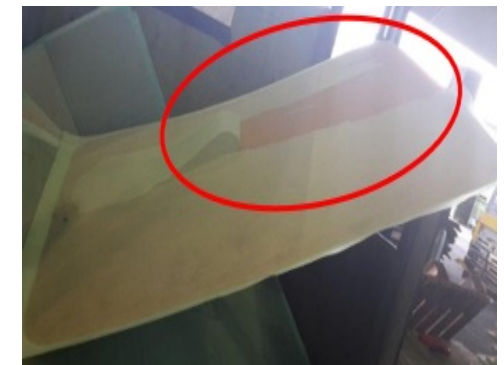
8. Recycle, missing foam
