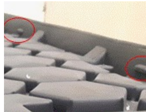
3. Lock-pins intact, if damaged repair
