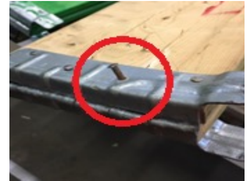
4. Repair, loose rivet
