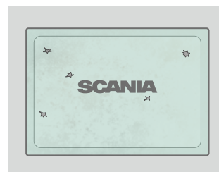
7. Multiple small holes
