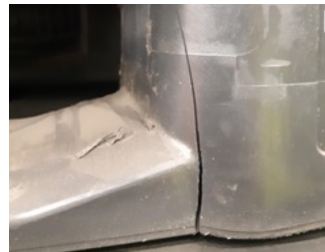
3. Recycle, large crack
