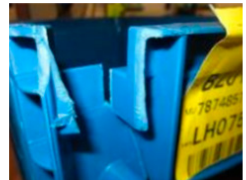
8. Recycle, broken corner
