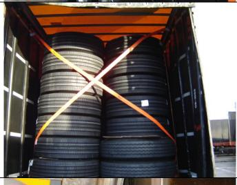
4 For the crossed belts use the lashing ring designed in the trailer.
