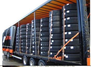
3 In the back the last piles are extra secured with crossed belts.
