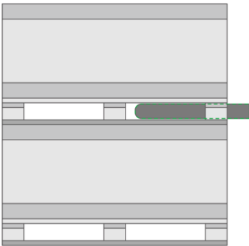
Figure 10 – Correct placement of forks
