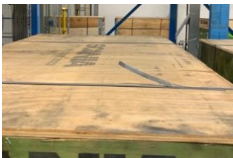
Figure 1 – Overlapping strap wich sticks out
