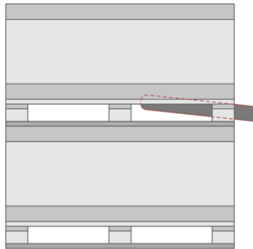
Figure 11 – Incorrect placement of forks
