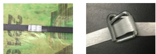
Figure 5 – Straps with metal connectors and nylon amplifiers shall not be used
