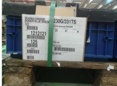
Figure 2 - Example of master label and strap not covering bar codes
