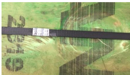
Figure 3 – Straps with metal connectors and nylon amplifiers shall not be used
