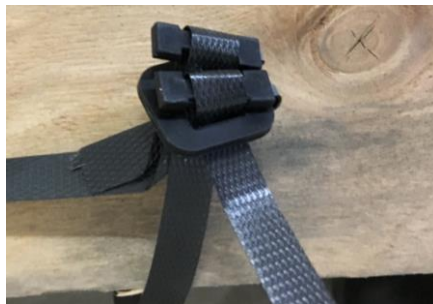
Figure 1 - Strap with connector from the same material as the strap
