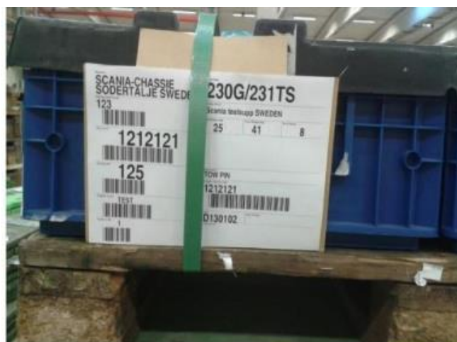
Figure 25 – Examples of master labels and straps not covering bar codes
