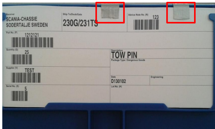
Figure 27 – VDA label inserted in the KLT holder and secured with e.g. adhesive dots/tape (as shown in the figure, see within the red squares)
