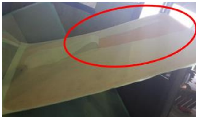
At least 10% of foam missing
