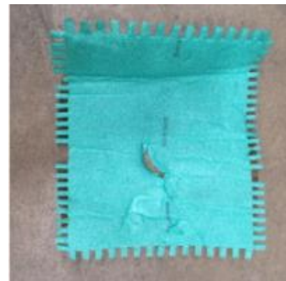
Holes straight through the spacer
