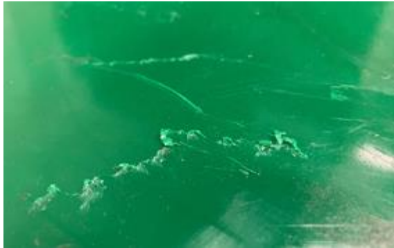
Scratches with unequal surface
