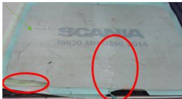
Cuts of more than 100mm must be scrapped
