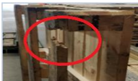
Broken, loose and/or missing Bottomboard/Runner
