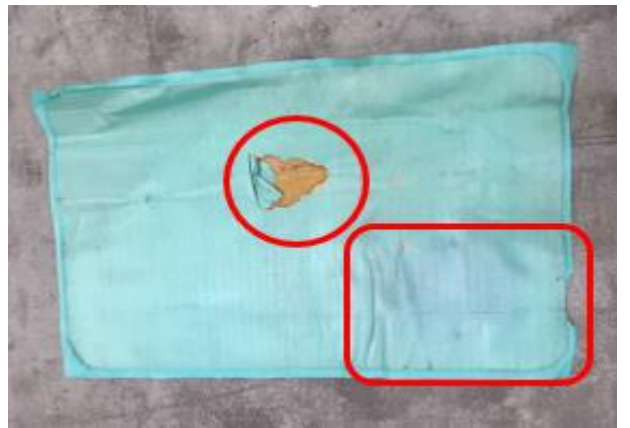
No damping is left in more than 10% surface area
