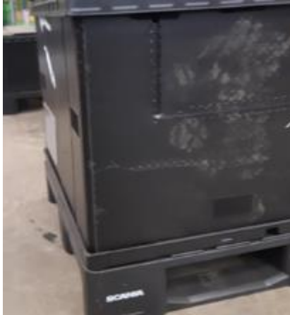
Sleeve needs wiping- visible dirt on sleeve
