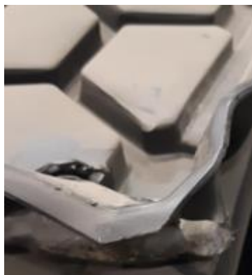
Crack through tray bottom
