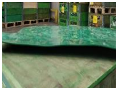
Bent more than 30 mm from its original straight shape
