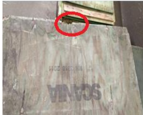
Damages left by straps
