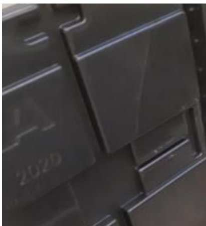
Lid with top crack, can let in dust or liquid
