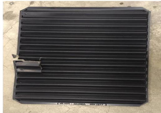
Example: Cracks bigger than 20mm
