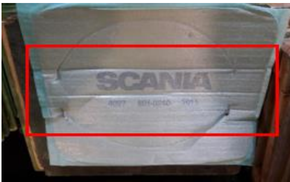
Out of shape, more than 40% on the surface area and can't regain its original shape
