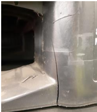
Large crack through runner. Needs to be recycled
