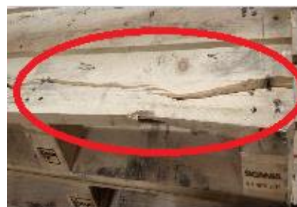
Broken, loose and/or missing Deckboard
