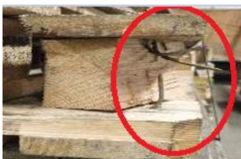
Pallets with protruding loose nails/screws
