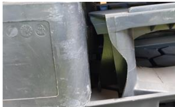
Runner broken. Needs to be recycled.
