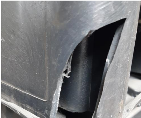
Crack in block but is OK since inner-block is not cracked.
