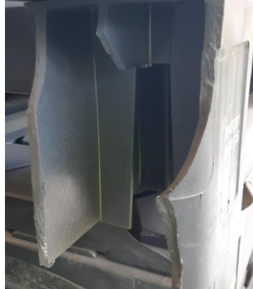
Crack completely through block. Needs to be recycled.
