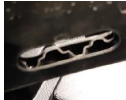
Picture of OK locking-hole. If damaged so it loses shape then recycle sleeve.
