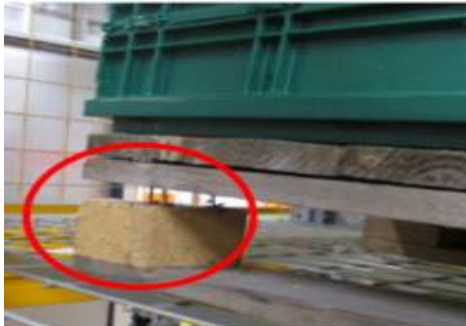
Broken, loose and/or missing Blocks
